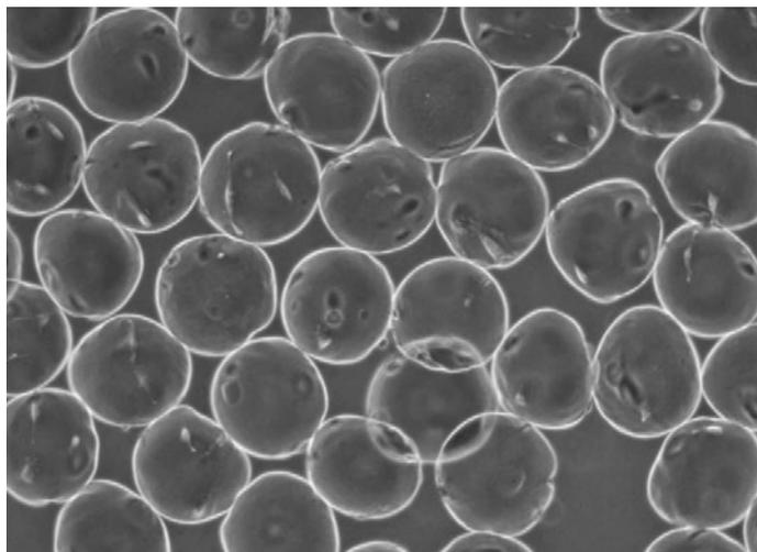
**Figure 2. hMSC attachment to Corning® dissolvable microcarriers after 5 hours.** Five hours after cell seeding, a 10 mL sample from the bioreactor was removed and transferred to an Ultra-Low Attachment (ULA) 6-well plate. Cell attachment and uniformity of distribution were assessed via microscopy. A representative image at 5X magnification is shown.
