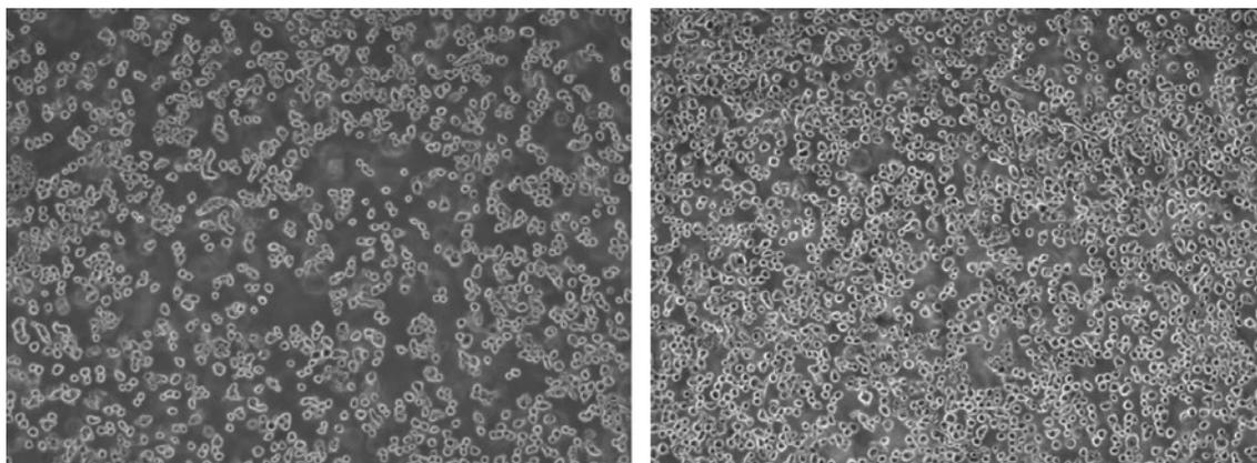
**Figure 7. Cell suspensions after microcarrier dissolution.** Microcarriers were dissolved in 5L bioreactors using a harvest solution of TrypLE, pectinase, and EDTA. Representative images of recovered hMSC suspensions post microcarrier dissolution are shown at 5X magnification.
