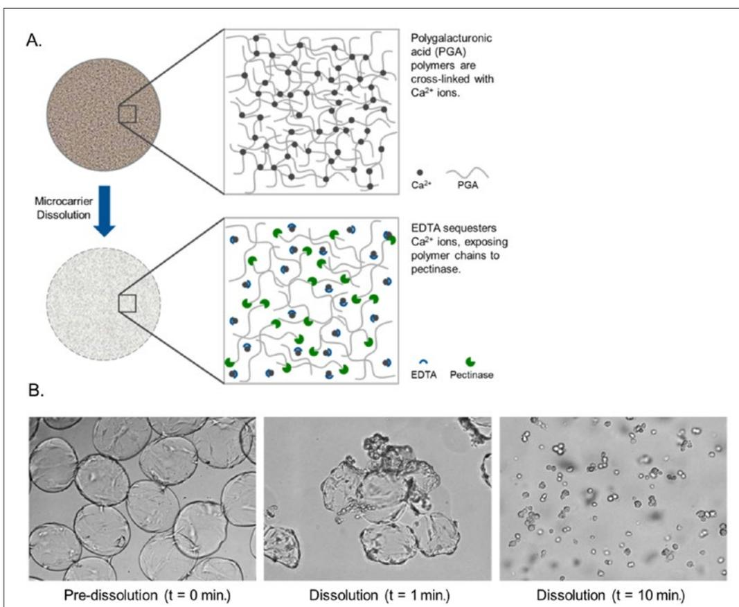
**Figure 1. Description of Corning Dissolvable Microcarriers.**
