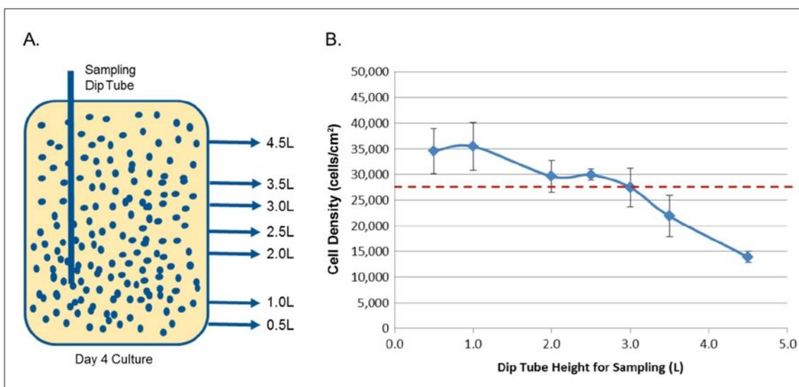
**Figure 6. Investigation of dip tube position for bioreactor sampling.** (A) Day 4 bioreactor cultures were sampled at various locations (or volume heights) within the bioreactor as shown by the position of the 7 blue arrows. (B) cells were enumerated from samples taken at these locations; error bars represent the standard deviation of 3 independent bioreactor runs. The average cell density across the 7 samples was calculated as 27,000 cells/cm<sup>2</sup> and shown by the red dotted line.
