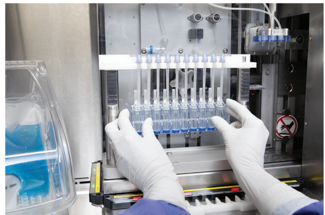
The CellSeal® SAFS-100 Semi-Automated Filling System in operation under a biosafety hood.
