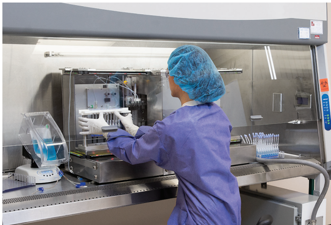
The CellSeal® SAFS-100 Semi-Automated Filling System in operation under a biosafety hood.
