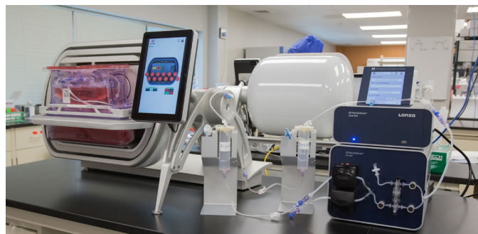
Figure 1: Cocoon® Platform integration to the 4D-Nucleofector® LV Unit via functionally-closed tubing connections. Standard Nucleofection® Process tubing set with the 4D-Nucleofector® LV Output Reservoir connected to the Cocoon® Platform
